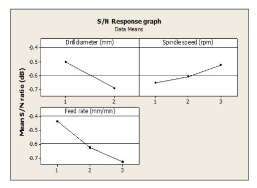
Fig.5: S/N Response graph for Delamination factor (effects of drill diameter)
