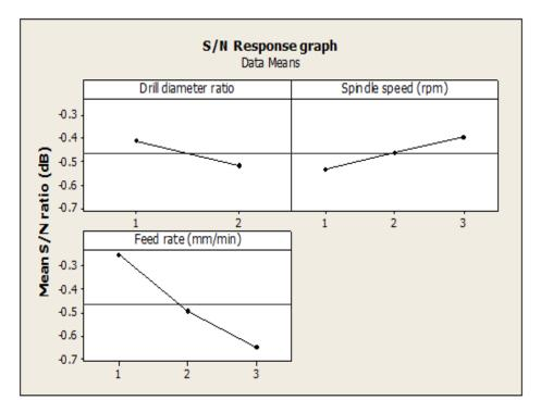
Fig.6: The S/N Response graph for Delamination factor (effect of drill diameter ratio)
