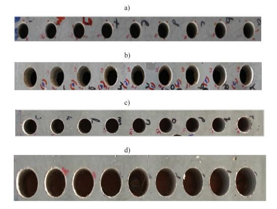
Fig.1: Drilled holes for delamination studies; a) Ø8mm drilled holes, b) Ø15mm drilled holes, c) Ø10mm holes obtained by drill diameter ratio of 0.8 and d) Ø15mm hole obtained by drill diameter ratio of 0.53
