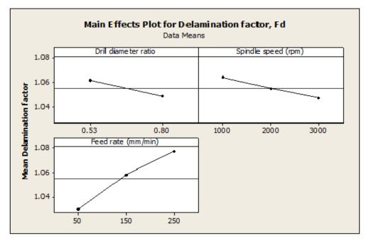
Fig.4: The main effects plot for Delamination factor (effect of drill diameter ratio)
